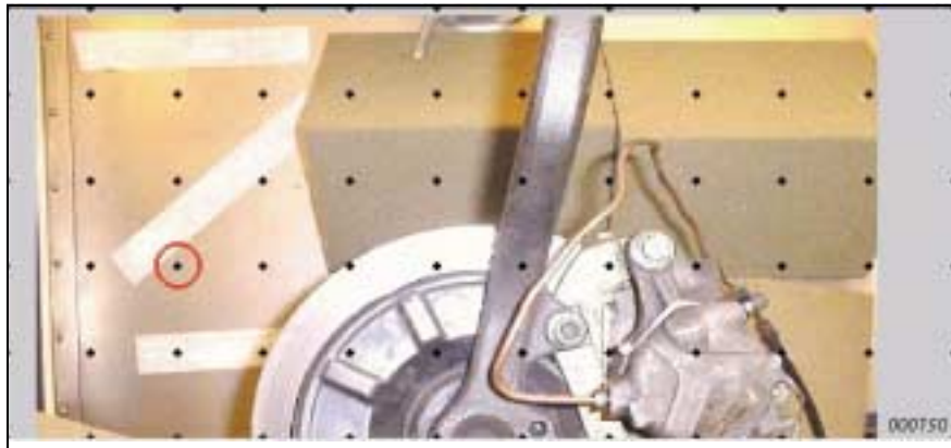
Fig. 1 Measurement area with indication of array microphone positions (dots).
