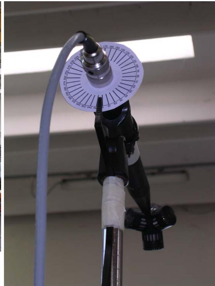
**84 IRs were measured, uniformly scattered around a sphere**
