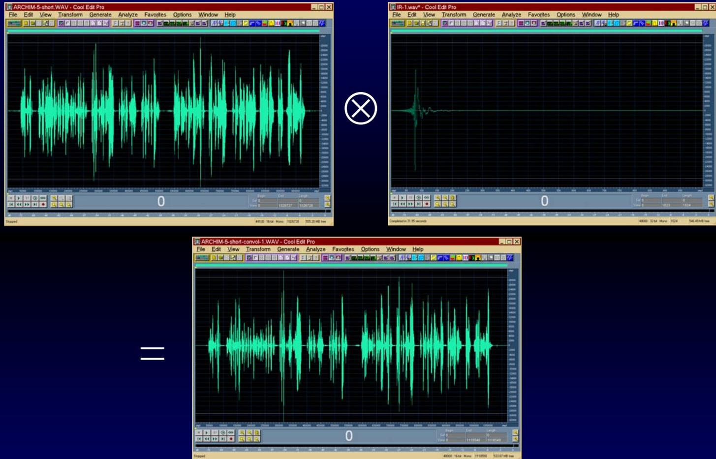
Convoluting linearly a suitable sound sample with the Imp.Resp., the frequency response and temporal transient effects of the system can be simulated properly
