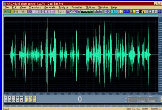
Convoluting a suitable sound sample with the linear IR, the frequency response and temporal transient effects of the system can be simulated properly
