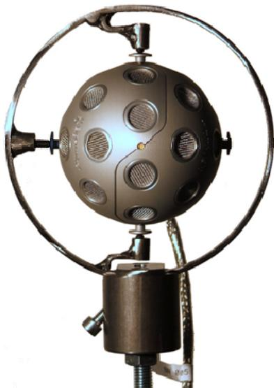
Subsequent rotations of the probe along a meridian, after selecting the meridian by manual rotation of the support.
