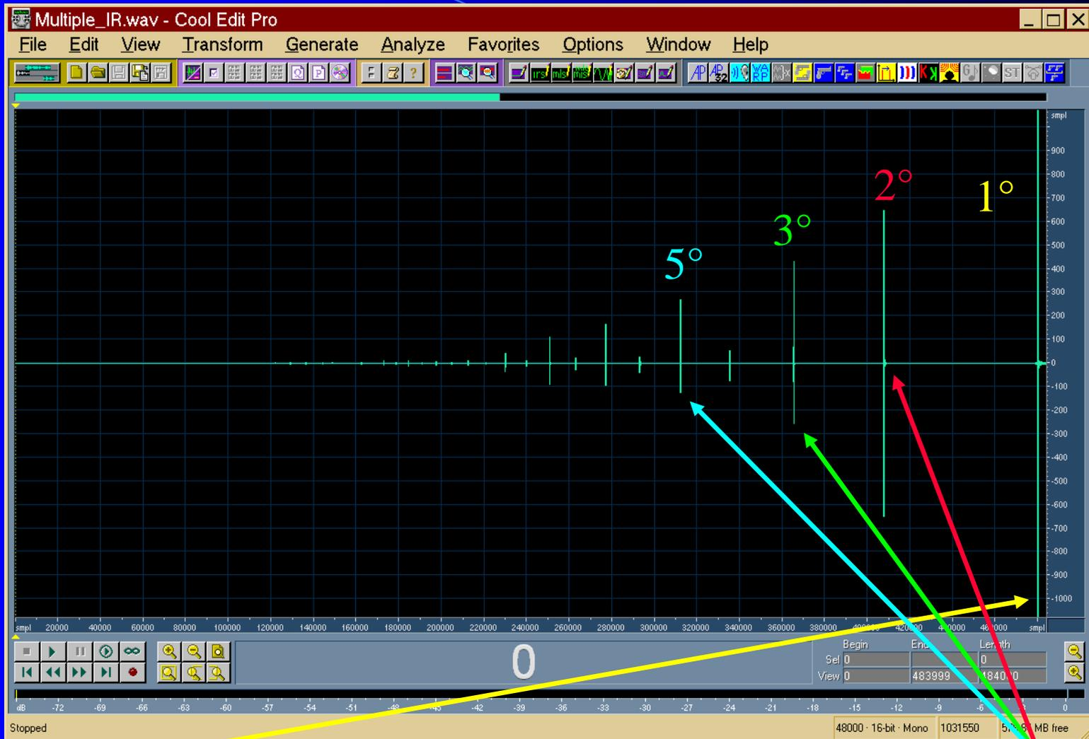
The last impulse response is the linear one, the preceding are the harmonics distortion products of various orders
