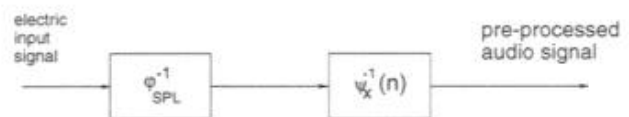
Fig. 9. Block diagram of an inverse filter effective for small displacements near an equilibrium position.
