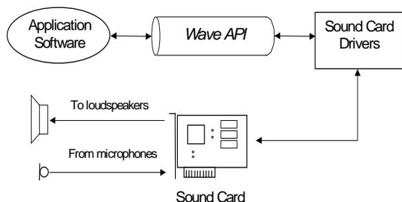
Figure 8. Sound system architecture
