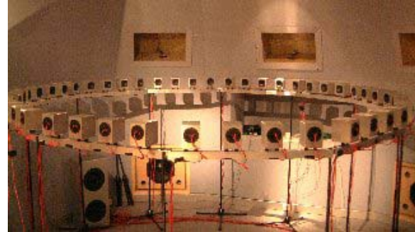
Figure 5 Quasi-circular 48-speaker array for WFS and HOA rendering experiments at the France Telecom R&D Labs
